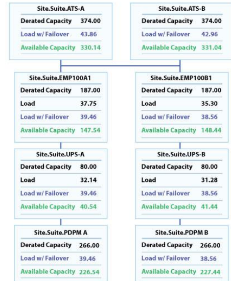
Figure 5: Cologix Command offers overall data center power consumption, detailing capacity and load figures for each equipment unit.
